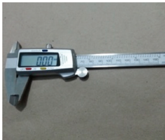
Figure 1. Calipers used for measurement of penile size in the newborn
